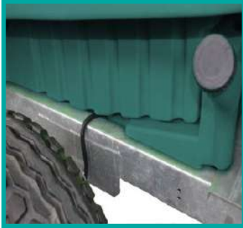
Serbatoio lava circuito Circuit washing tank
